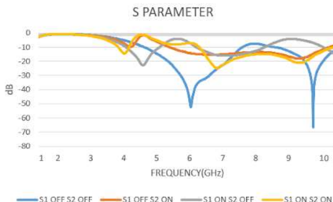
Fig. 4. S-parameter Analysis for Various Pin Diode Configurations
